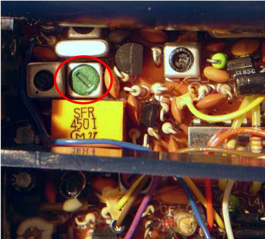
The ceramic filter SFR4501 is different than what we expected and has a distinctively small bandwidth of only  $\pm 2$  kHz and rather steep edges. While yielding an very good selectivity for AM baseband signals, this means, that option a) would fail for DRM, as we need a bandwidth 8 kHz or so. Yet, this also means that we cannot use the pre-amplified IF.
