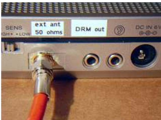
The 12 kHz DRM output signal will be hooked to the "line out" jack socket labelled with a tape symbol. The original audio output signal will be disconnected, as it is not of much use anyway. The signal is far below specs for "line out".
